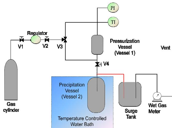
Figure 2: The schematic diagram of the DESAM system
